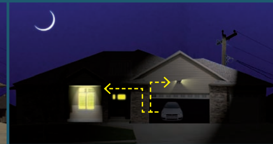
Lack of network: the EV works with a no-break that ensures energy supply.
